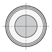
$\begin{array}{ll} d1 & = 18 \\ d2 & = 14 \\ h & = 8.0 \\ Holding force N = 10 \end{array}$
